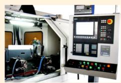
The machines are designed for simultaneous grinding of plunge grinding of several diameters & shoulders without change in setups. All the operations are done in a single setup using a formed wheel or multiple wheels that help in accurately controlled profile geometry & contributing to increased productivity.
