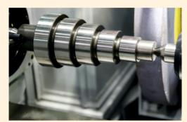
The machines are designed for simultaneous grinding of plunge & traverse grinding of several diameters without change in setups. All the operations are done in a single setup using a formed wheel or multiple wheels that help in accurately controlled profile geometry & contributing to increased productivity.
